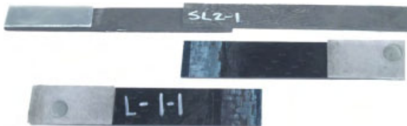
Fig. 7. Single-lap shear element-level test for the adhesive, before (top) and after failure (bottom).
