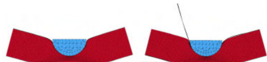
Fig. 20. Comparison between the morphologies of the simulation of the assembly at the end of the penetration test for the case with the measured adhesive strengths (left), the other with the reduced set of strengths (right).
