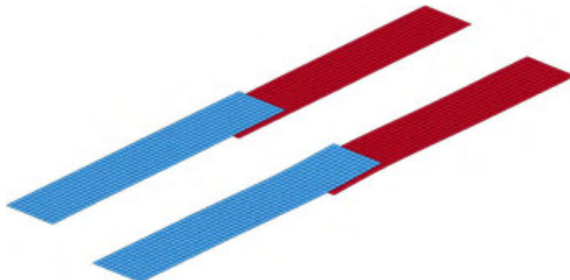
Fig. 15. Single-lap shear simulation of the adhesive, at the beginning (left) and the end (right) of the loading.
