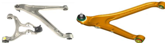
Fig. 3. Front upper and lower aluminum arms (left) and CAD detail of front lower arm (right).
