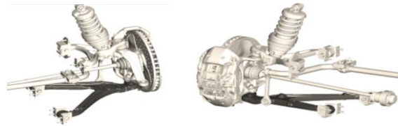
Fig.2. Two views of the wheel assembly showing front lower and upper control arms.
