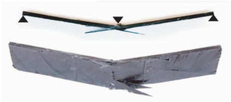
**Figure 25.** Flexure specimen failing in tension directly below the loading roller.
