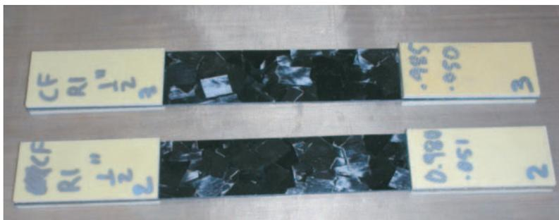
**Figure 4.** Typical tensile test specimens with glass fiber/epoxy tabs.
