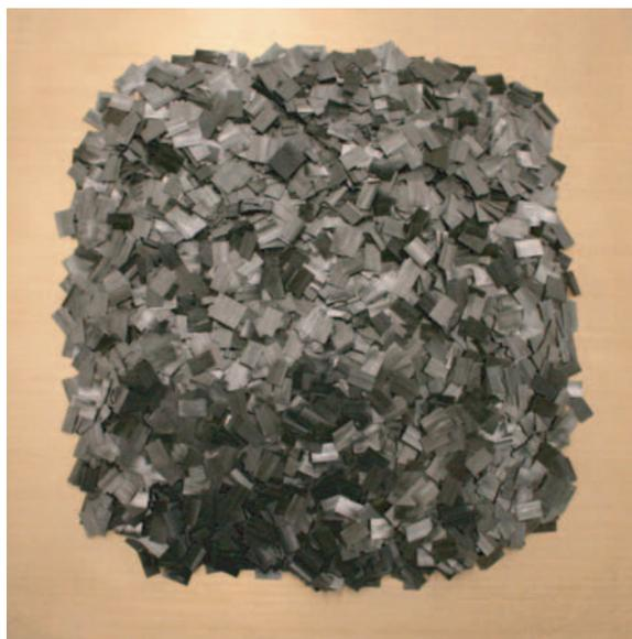
**Figure 2.** Random distribution of prepreg chips before curing.
