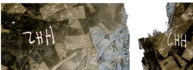
Fig. 4. Failure surface of UNT specimen shows extensive fiber failure.
