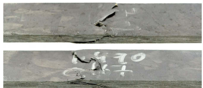
Fig. 12. Representative UNC specimen failure morphology (left and right sides).
