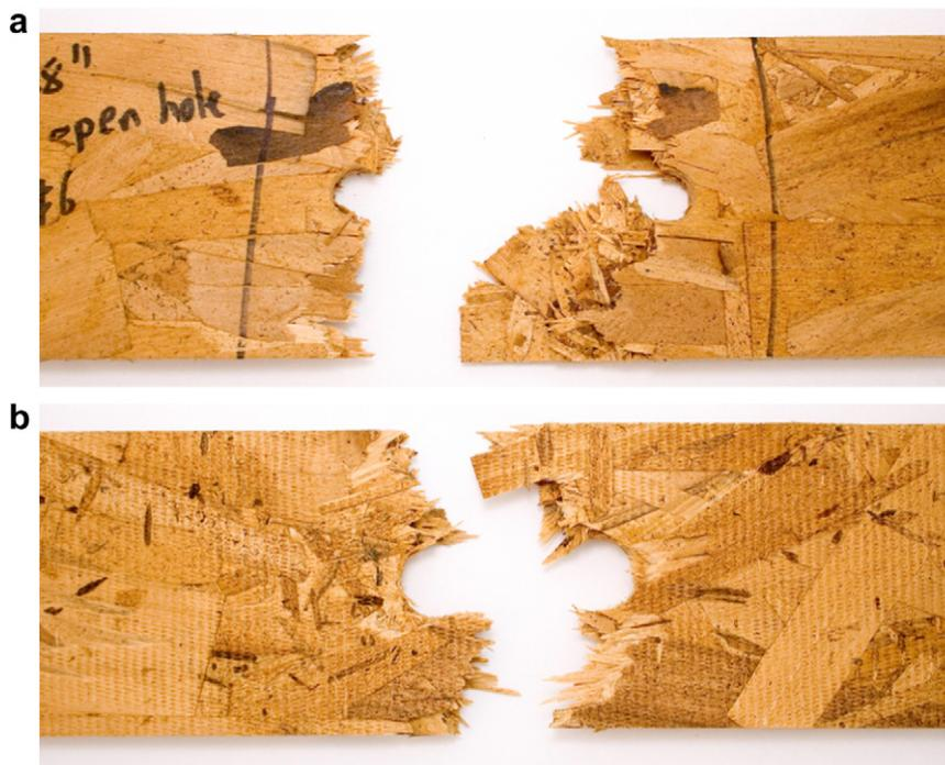
Fig. 5. (a, b) OSB specimens show failure at the net section for (a) 0.50 in. (12.7 mm) and (b) 0.75 in. (19 mm) diameter holes.
