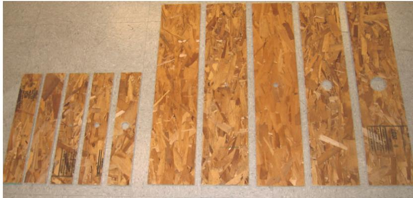
Fig. 1. Examples of baseline OHT specimens and scaled-up specimens with various hole diameters.
