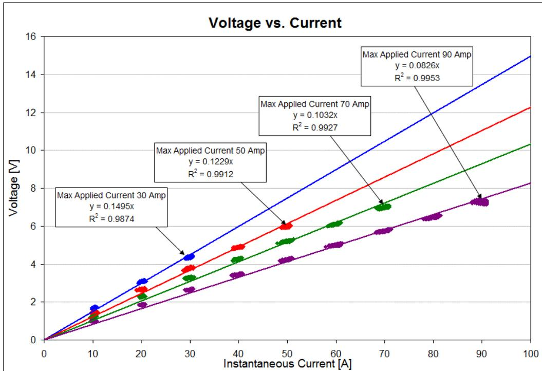
Figure 3. Voltage vs. Current Characteristics of a CFRP Laminate
