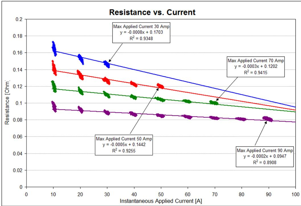
Figure 4. CFRP Resistance vs. Current
