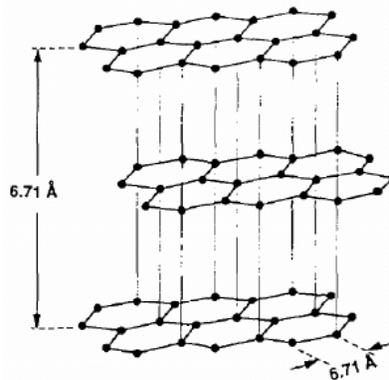
Figure 10. Hexagonal arrangement of carbon molecules.
