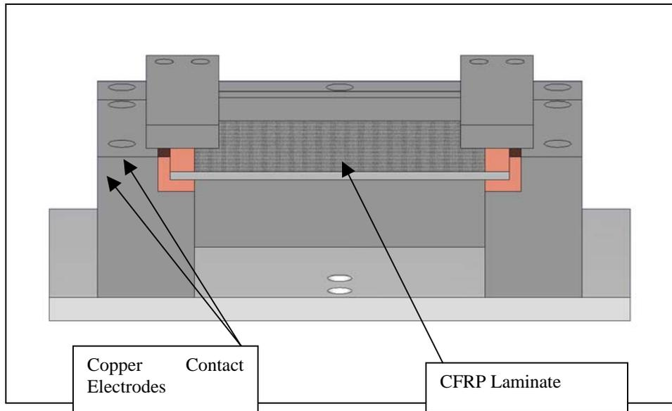
Figure 1. Cross-sectional illustration of the test fixture
