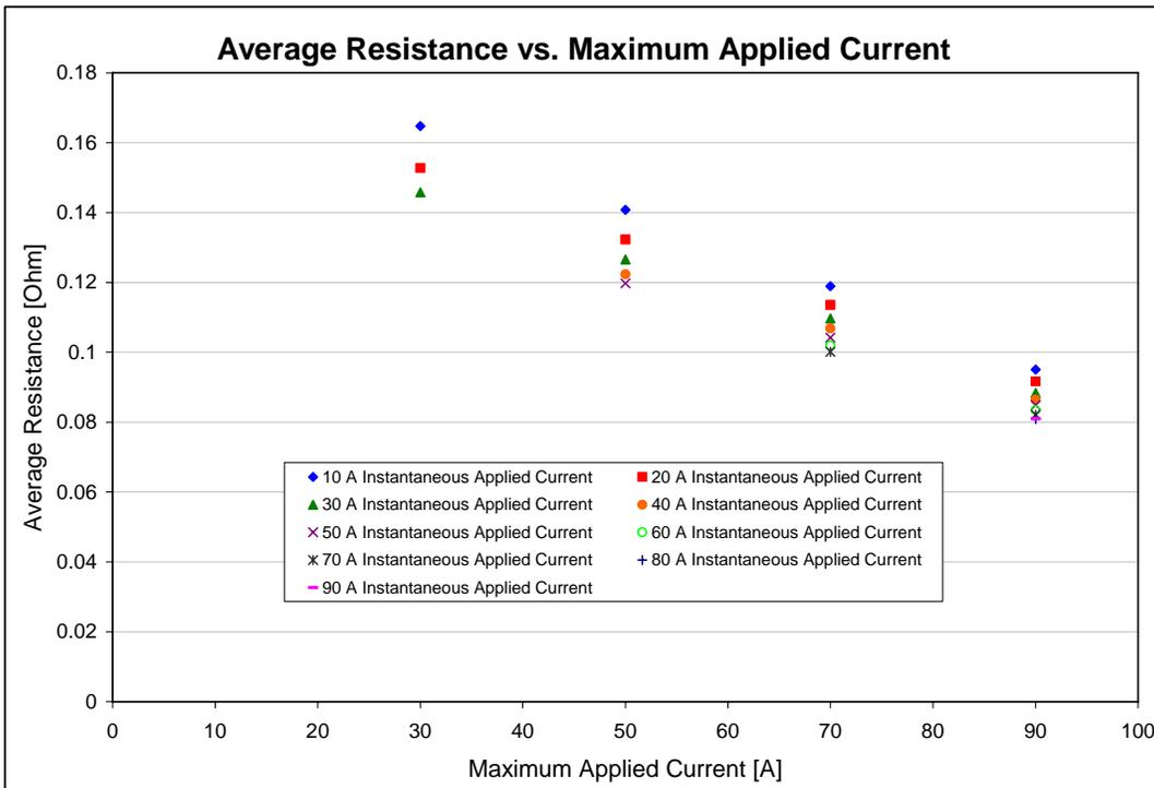
Figure 5. Average Laminate Resistance vs. Maximum Applied Current
