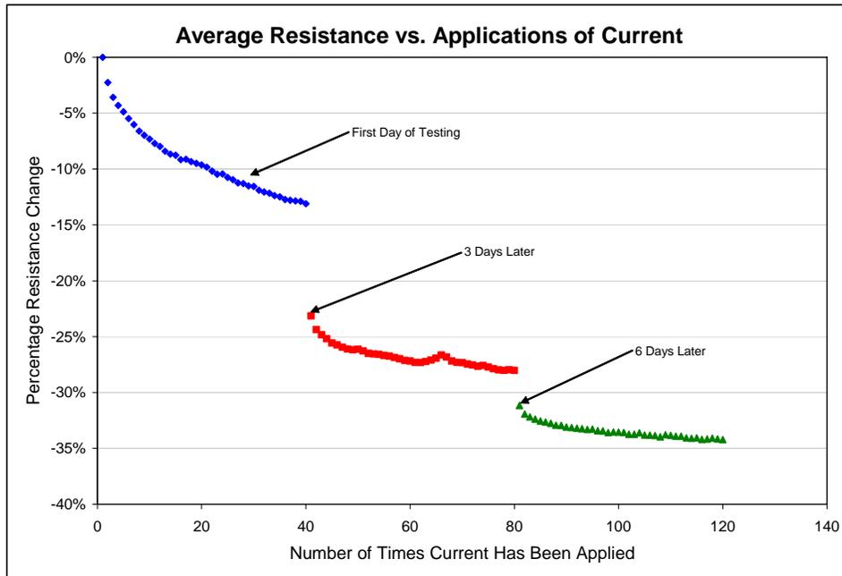
Figure 6 a and b. Percent Change in Laminate Resistance vs. Number of Times that a 30 Amp current is Applied a) in one day, b) after 3 and then 6 days
