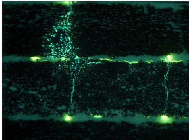
Figure 9. Micrographic picture of an interlaminar area of the plate after electrification.
