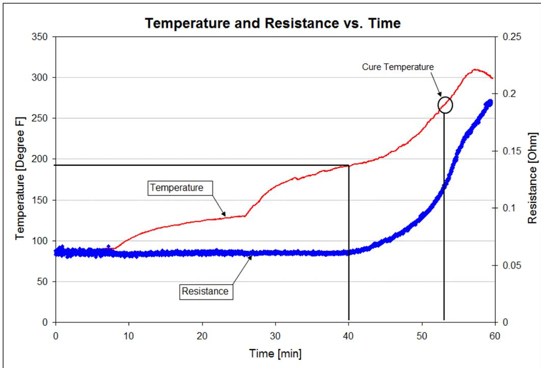
Figure 8. CFRP Laminate Surface Temperature and Resistance vs. Time
