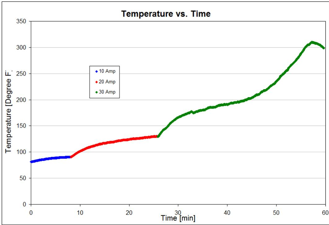
Figure 7. Surface Temperature of CFRP Laminate vs. Time
