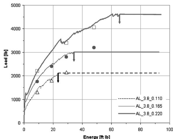
**Fig. 12 Force–energy curves obtained by quasi-static indentation and superimposed force–energy impact test data points showing analogy between quasi-static and low-velocity events for carbon/epoxy systems.**
