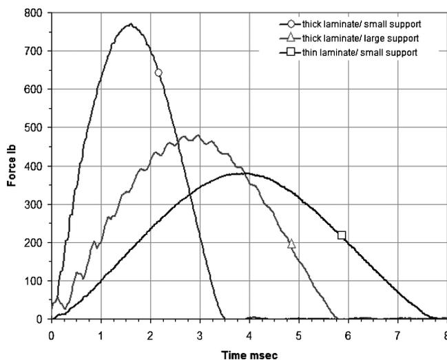
**Fig. 4** Three impact tests performed at the same energy level (1 ft · lb) on three different laminate thickness/support span combinations: a) 32 ply  $t$  on 2.5-in.-diam aperture  $D$ , b) 32-ply  $t$  on 5-in.-diam aperture  $2D$ , and c) 16-ply  $t/2$  over 2.5-in.-diam aperture  $D$ .
