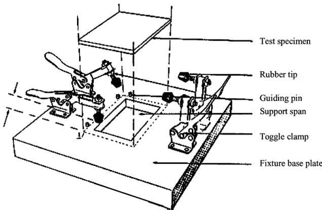
Fig. 6a Impact support fixture with four clamps.
