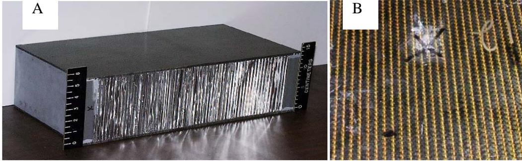
Fig. 2 A, B. Sandwich panels used in the present investigation, having dimensions 20 in. x 10 in. x 5.5 in. (A), and close-up of the stitched CFRP skins (B).
