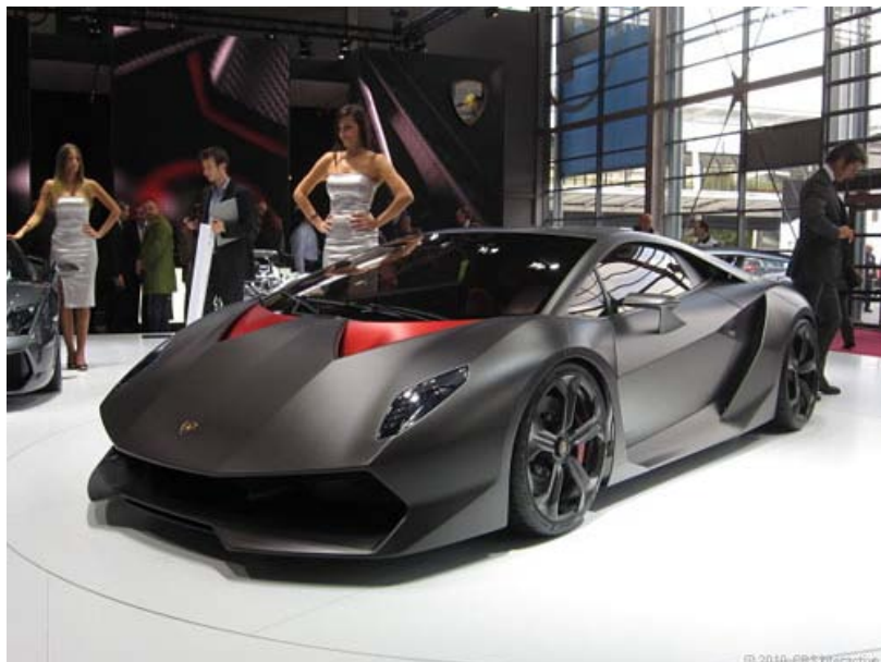
Lamborghini unveiled the Sesto Elemento concept at the Paris auto show. Many body parts and structural components use carbon fiber. Even the car's tailpipe is made from a carbon and glass-ceramic composite.
