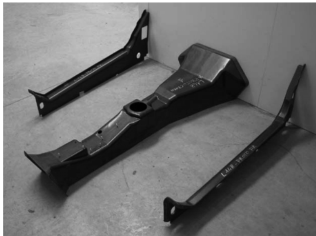
Figure 7 New CFRP structural components on the Roadster include an elongated transmission tunnel and the door sill stiffeners
