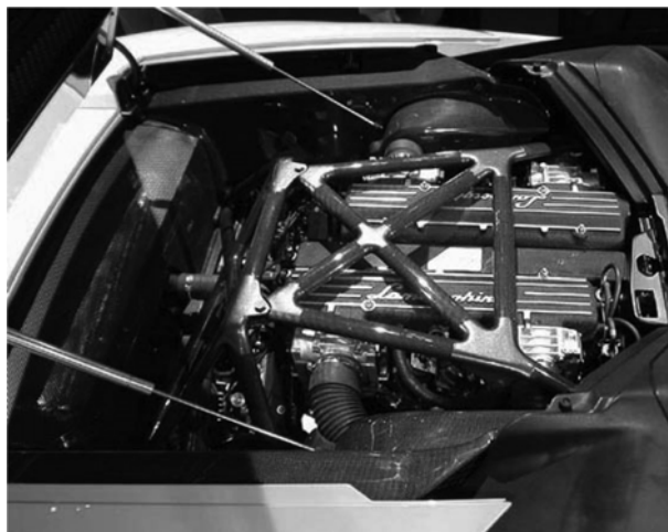
Figure 8 The engine bay subframe, featuring transparent CFRP struts and titanium-coloured CFRP joints
