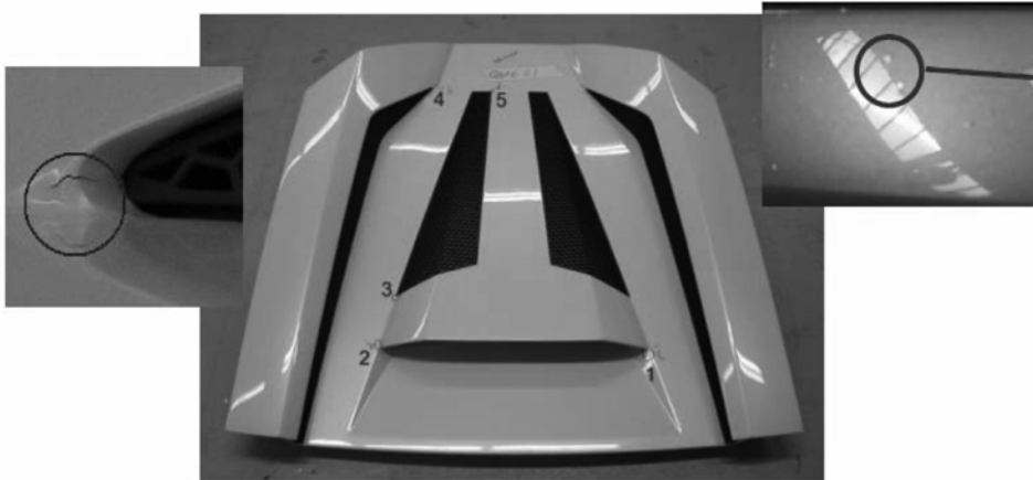
Figure 6 Typical blistering and cracking problems that can be observed in the manufacturing of class A components with complex geometries and large surfaces
