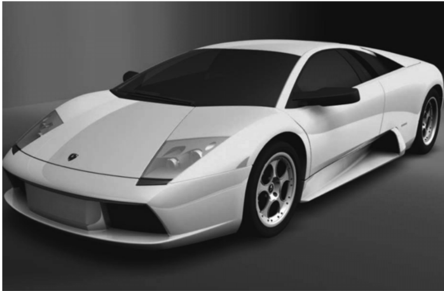
Figure 1 The CFRP body components of the murcièlago include the four fenders, the front and rear bumpers, the large rocker panels, the variable geometry air intakes, the front hood and the rear engine bonnet
