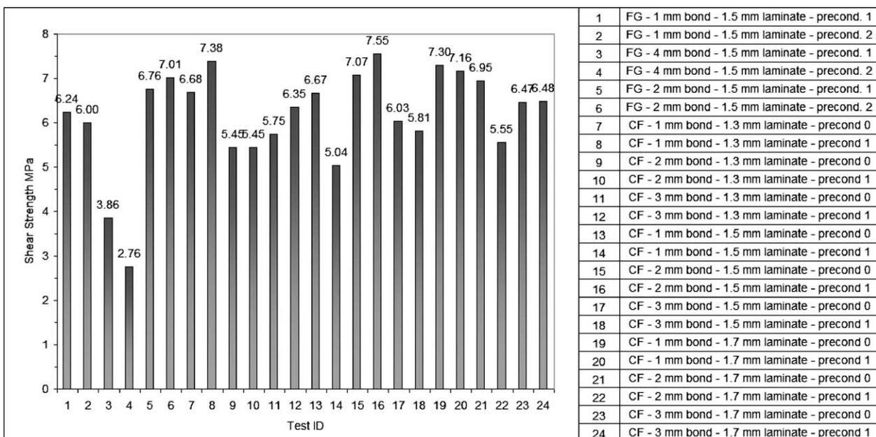
Fig. 7. Bonded joint shear strength for carbon and glass fiber adherents for four values of bond-line thickness; three values of laminate thickness; three types of environmental preconditioning.
