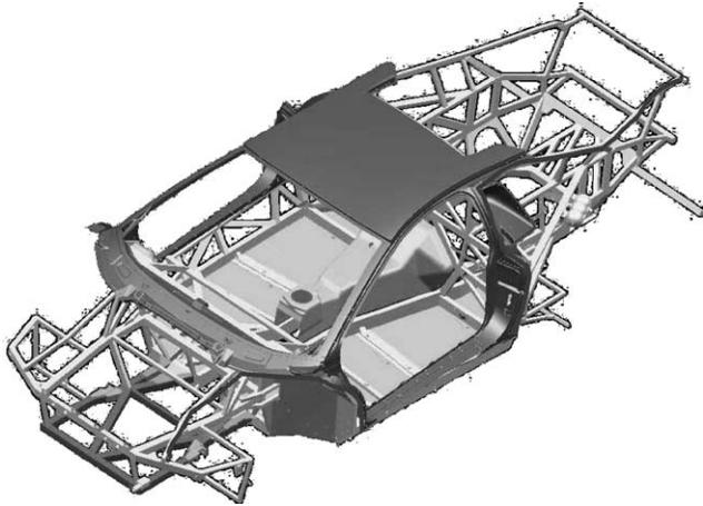
Fig. 8. Tubular chassis and passenger compartment of the Murcièlago. Light blue indicates the carbon/epoxy floor pans, rocker panels and transmission tunnel. The red lines represent the rails along which body panels are adhesively joined to the frame.
