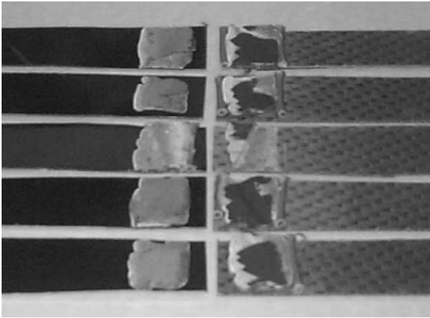
Fig. 6. Single lap shear test coupons: EPC steel adherent on the left and carbon fiber on the right. Visible are also the blue paste of the methacrylate adhesive and the red spacing wires. All three failure modes are visible.
