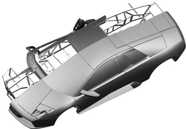
Fig. 1. The composite body of the Murcièlago is shown over its tubular steel frame and steel roof structure.
