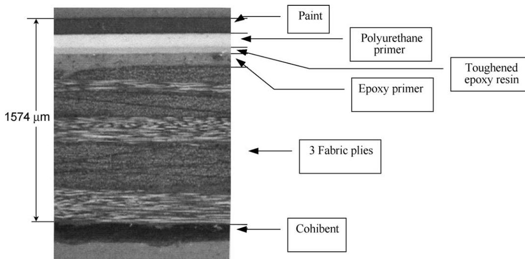
Fig. 4. Micrographic cross-section of body panel.
