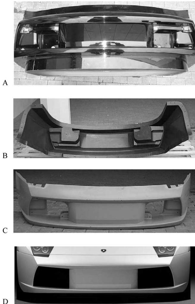
Fig. 5. (A) Epoxy model for the front bumper: visible is the black epoxy finish for surface inspection; (B) Graphite/epoxy mold obtained from the previous model; (C) Component after extraction from the mold: visible is the green epoxy primer for better paint absorption and sanding; (D) Final component after painting and assembly.
