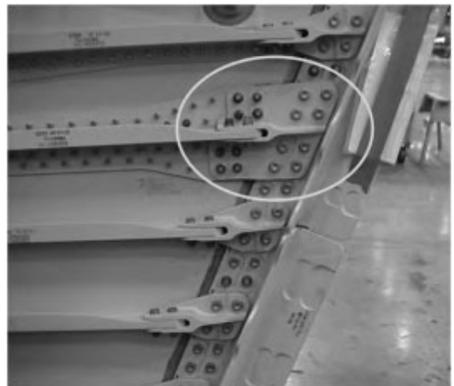
Fig. 13 Skin/stringer-to-root fitting considered for this case study.
