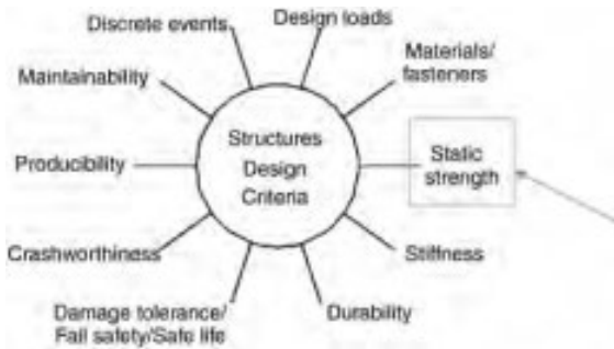
Fig. 1 Design drivers for composite structures, highlighting the focus of the paper on static strength requirements.
