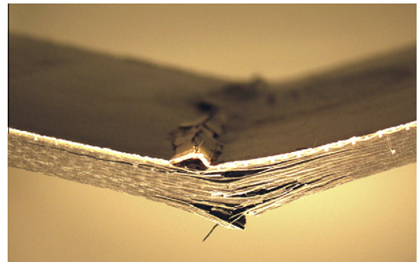
Fig. 23. Typical flexural failure, with tensile fiber breakage on the lower side and compressive kinking of fibers and copper mesh on upper side. (For interpretation of the references to color in this figure legend, the reader is referred to the web version of this article.)
