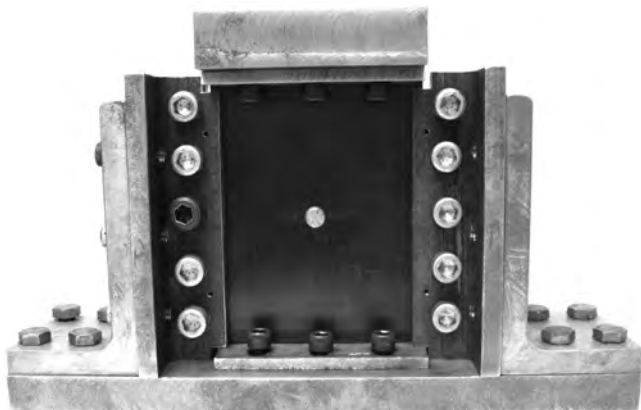
Fig. 24 CAI test fixture with filled-hole specimen following lightning strike damage.
