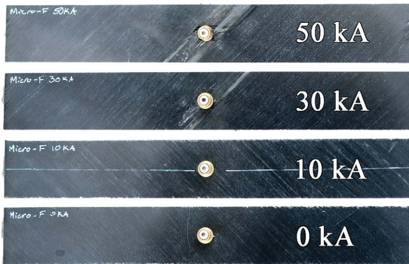
Fig. 13. Typical filled-hole specimens, from pristine at the bottom to maximum current at the top.
