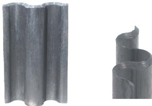
Figure 8. Corrugated Test Specimen With 45° Single-Sided Chamfer Trigger
