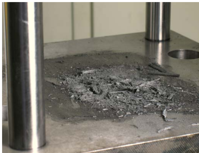
Figure 13. Carbon Fiber/Epoxy Dust and Debris Left in the Test Fixture Following a Crush Test
