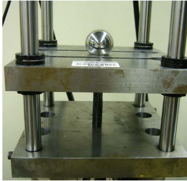
Figure 9. Test Fixture With Specimen Installed
