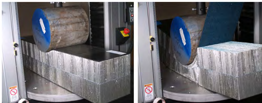
Fig. 8. Subcomponent level test of the full assembly being penetrated by the pole at two different instants during the test.
