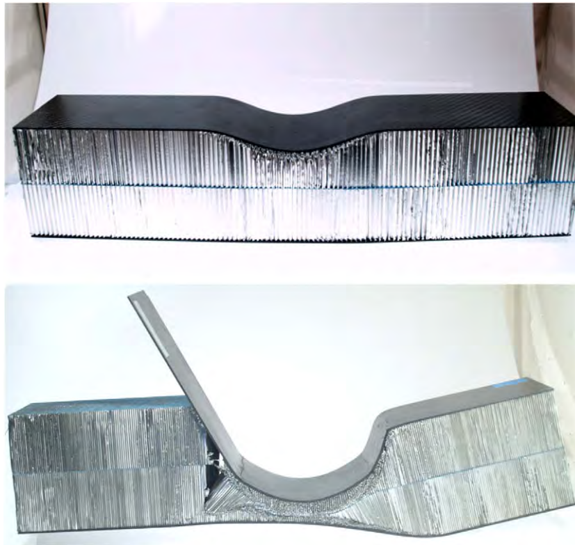
Fig. 9. (Top) Partially crushed morphology of the assembly – test was interrupted to take picture. (Bottom) Final morphology of the assembly after testing.
