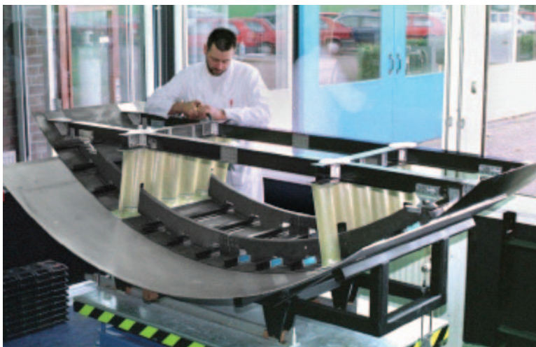
Figure 1. Composite-intensive study of energy-absorbing subfloor of commuter aircraft [8].
