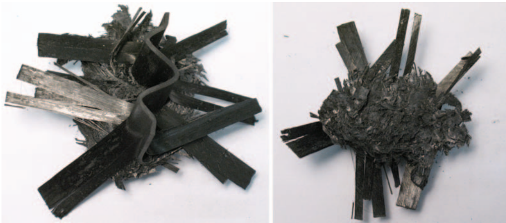
Figure 20. Top and bottom view of crushed specimen for configuration 2.
