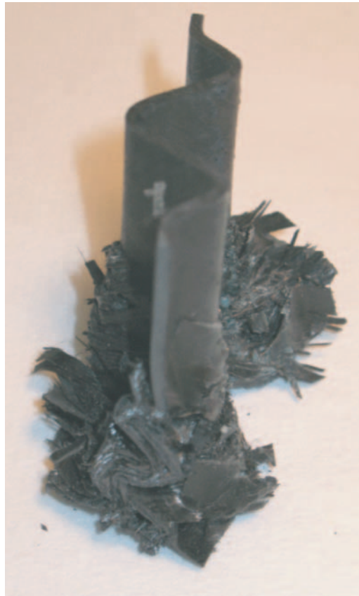
Figure 16. Local buckling of the fronds for configuration no. 5.
