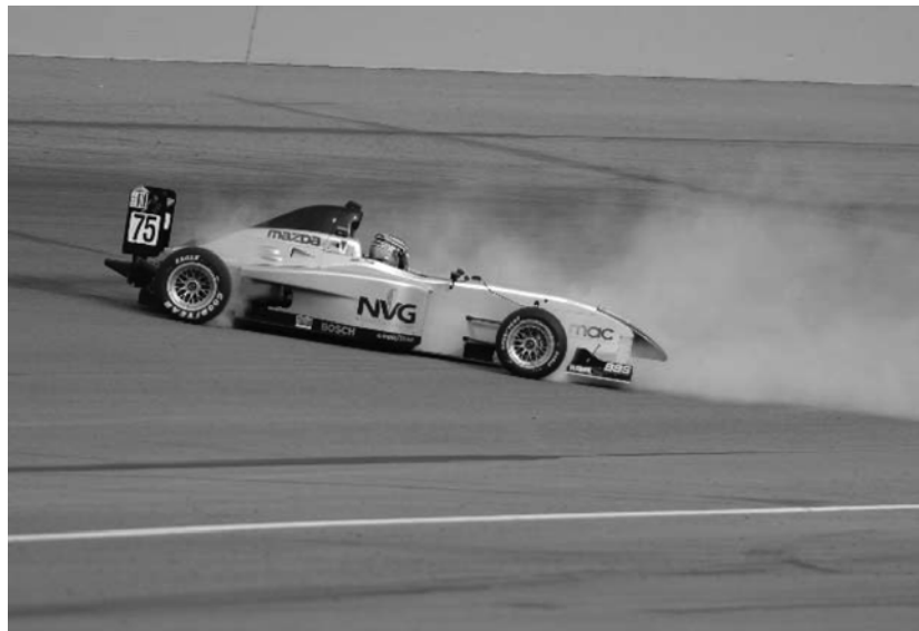
Figure 1 Typical Star Mazda Championship racecar photographed after losing control on the oval racetrack and while spinning towards the wall. The CFRP RIMP is visible in the aft portion of the vehicle below the wing
