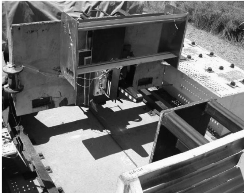
Figure 5 Crash test setup showing the RIMP/gearbox/wing assembly and the impacting plate mounted on the moving sled
