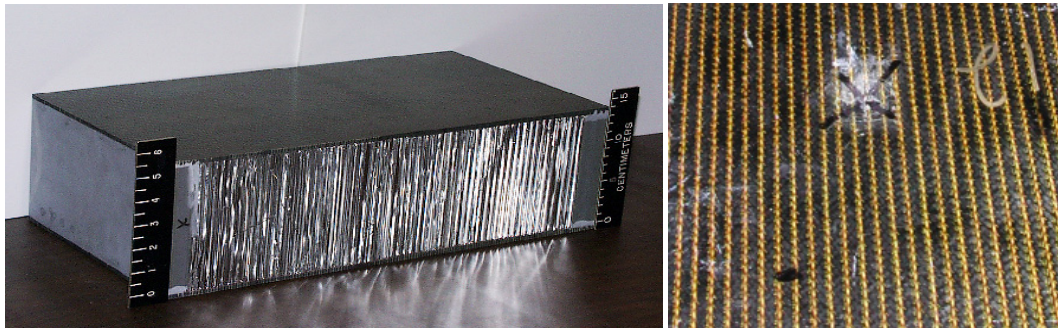
Figure 1. Sandwich panels used in the present investigation, having dimensions 20 in. x 10 in. x 5.5 in., and close-up of the stitched CFRP skins.
